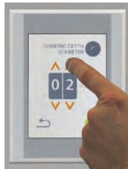
Step 4. Set grind amount (in increments of 0.001" or 0.01mm)
