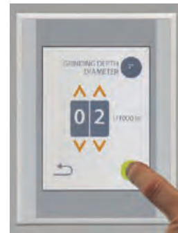
Step 5. Touch start to sharpen the tool
