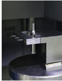
Step 1. Load tool into chuck
