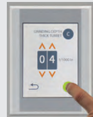
Step 5. Touch start to sharpen the tool.
