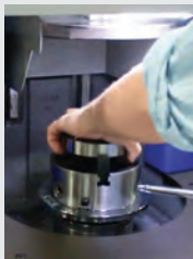
Step 1. Load tool into chuck.
