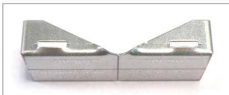
Component formed using conventional Air bending die.
