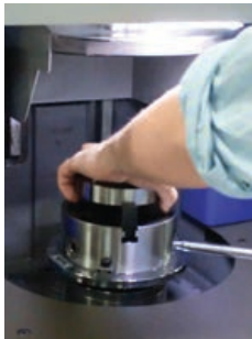
Step 1. Load tool into chuck
