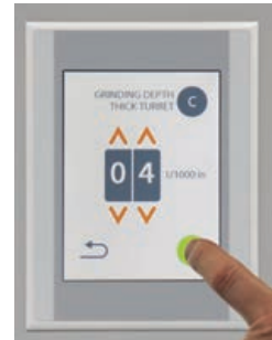
Step 5. Touch start to sharpen the tool
