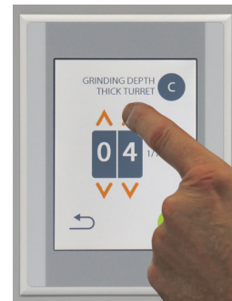
Step 4. Set grind amount (in increments of 0.001" or 0.01mm)
