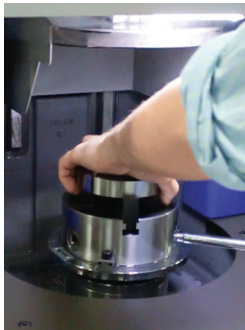
Step 1. Load tool into chuck
