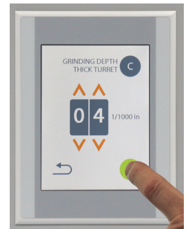
Step 5. Touch start button to sharpen the tool
