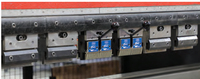
Add Express Clamps to your press brake wherever you need more efficiency. Holders are height compatible with OEM holders and can be placed in the middle of the press brake.
